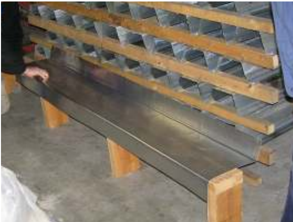
Cutting to size Lengths max. 3-4 metres.
