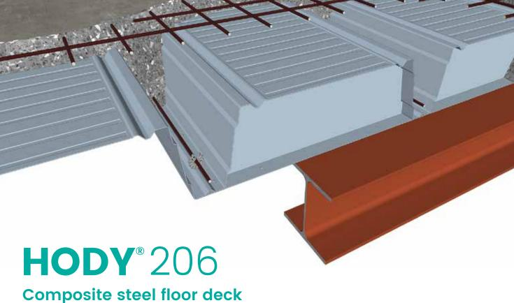
HODY 206 profiled steel sheets are used to create deep composite floor decks with a thickness from 260 mm. With this floor system it is possible to realise long spans up to 5990 mm without using temporary propping.
