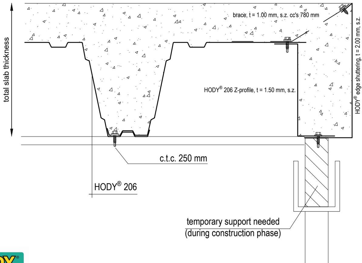
**HODY® 206** - detail 10 (longitudinal support with edge shuttering)
