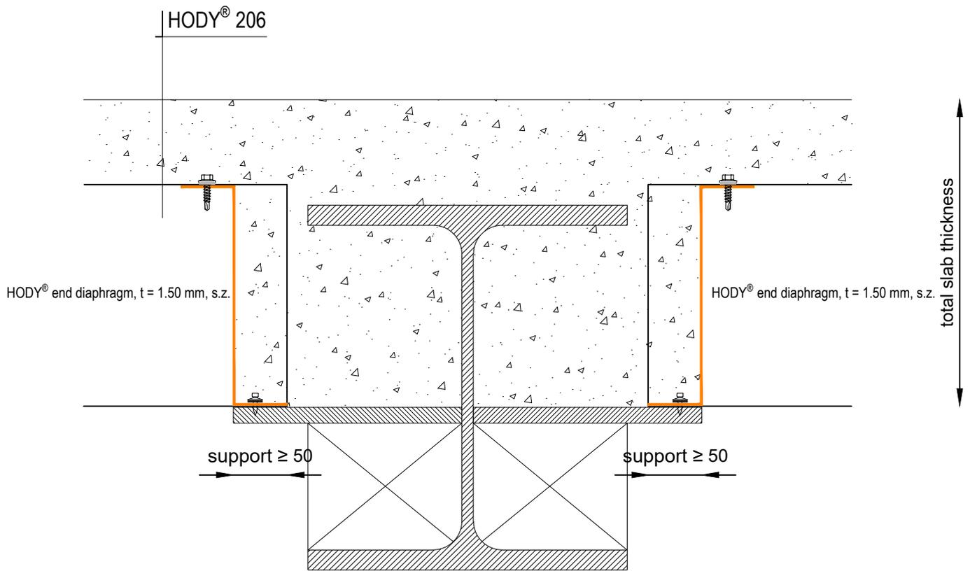
**HODY® 206** - detail 5 (end support in between the beam)
