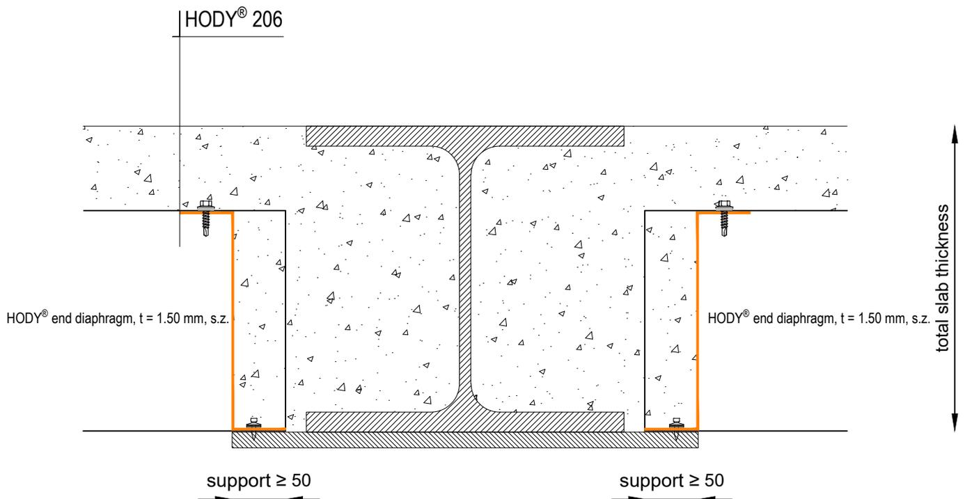
**HODY® 206** - detail 6 (end support with edge shuttering)
