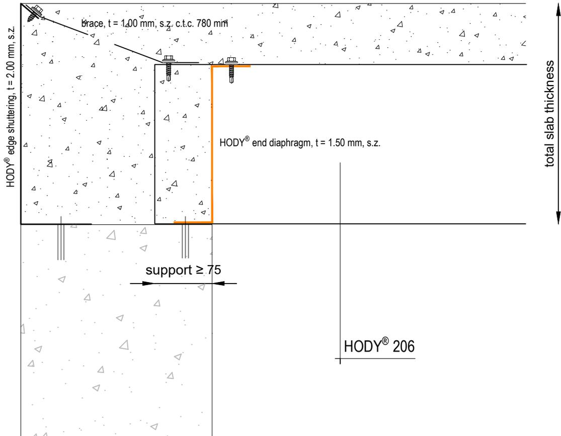
**HODY® 206** - detail 7 (longitudinal support with edge shuttering)
