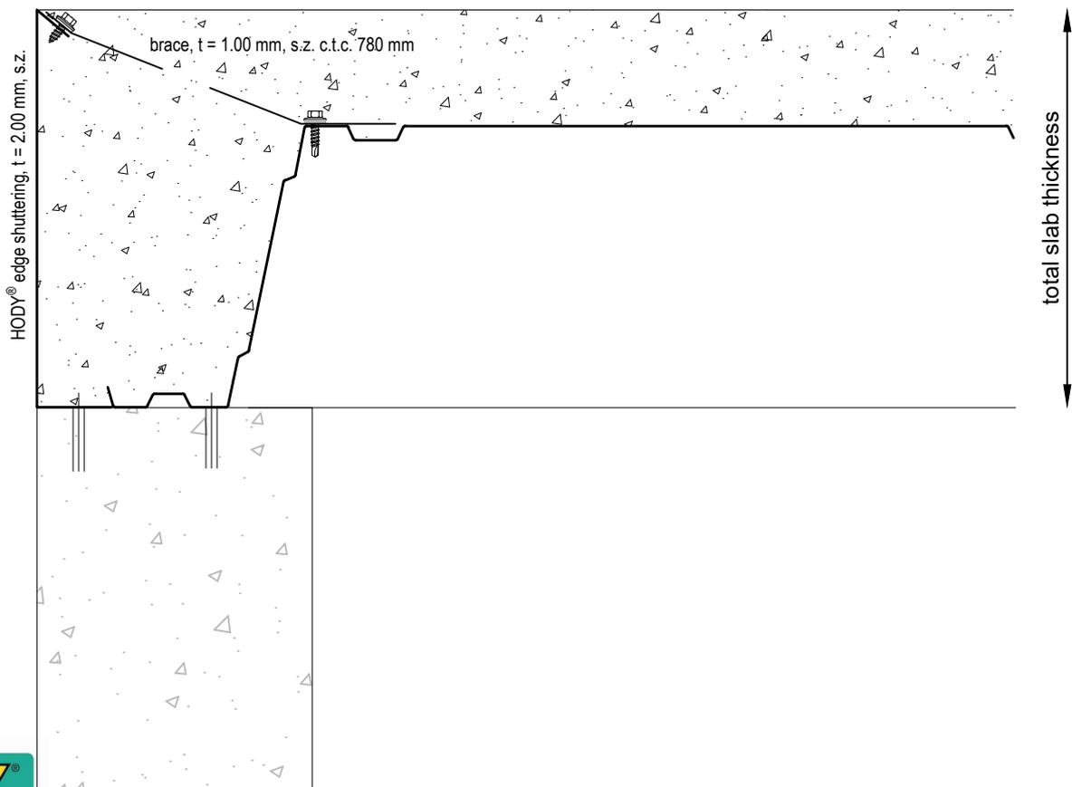
**HODY® 206** - detail 8 (longitudinal support with edge shuttering, propped)
