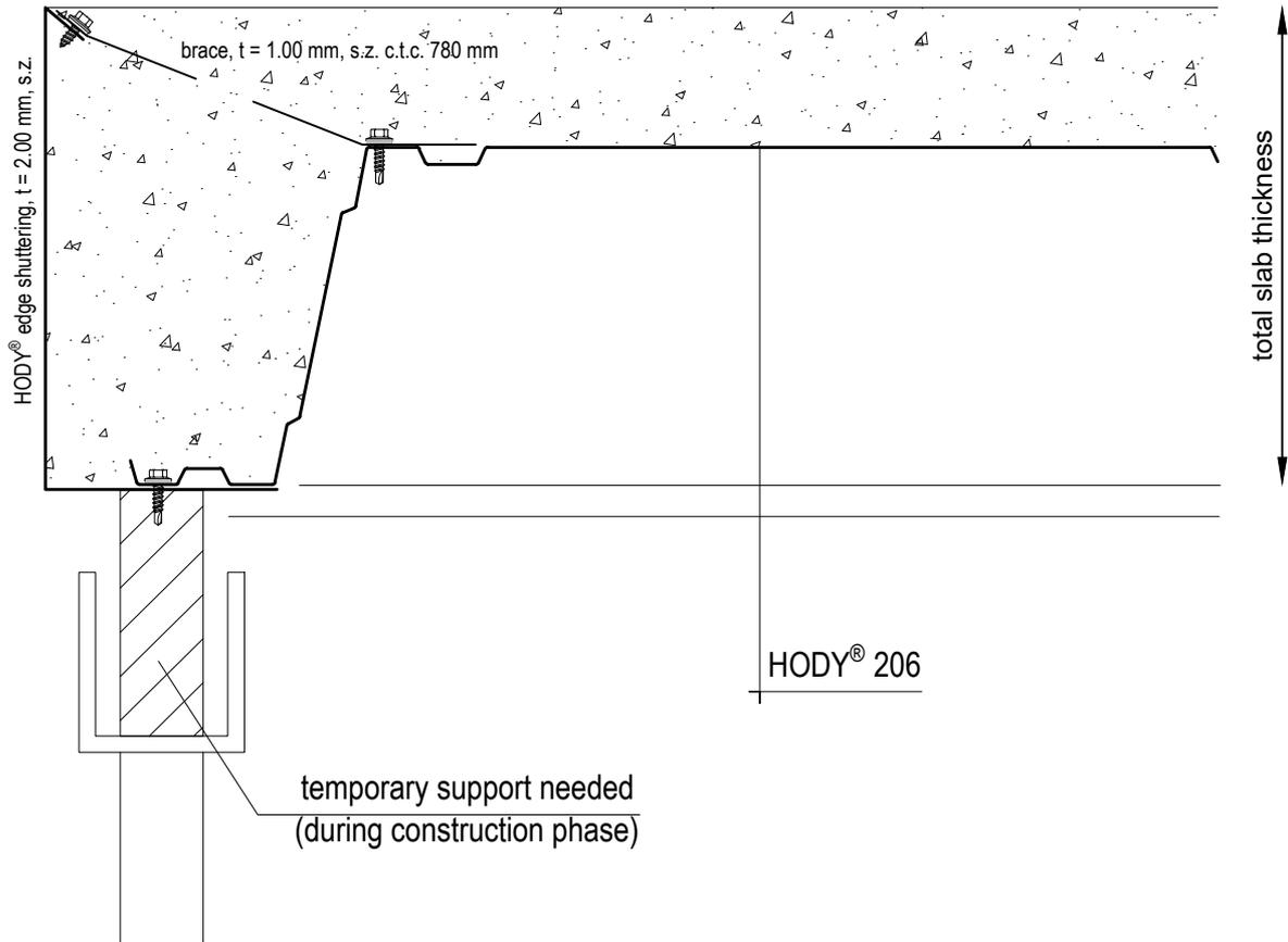
**HODY® 206** - detail 9 (longitudinal support with edge shuttering, propped)
