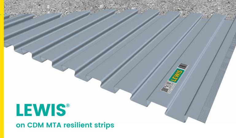
LEWIS® Dovetailed metal decking is used as reinforcement and formwork in thin concrete floors that are placed on wooden beam layers and light steel structures. The sheeting is finished with a thin layer of fine grade aggregate concrete or a screed. The composite action between LEWIS® Dovetailed metal decking and the concrete/screed ensures a rock-solid LEWIS® floor.
