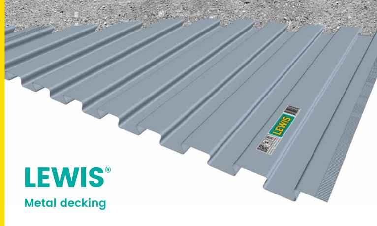
LEWIS® metal decking is a selfsupporting, light gauge galvanised steel reinforcement sheet, used for shuttering and reinforcing lightweight concrete or screeded floors of limited thickness (50 mm). Used in a composite floor construction LEWIS® Dovetailed metal decking provides a first class solution for fire protection, acoustic issues and Under Floor Heating & Cooling within floors.
